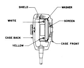
The Shure Model R103 is a direct replacement cartridge for the Shure Model 514B Omnidirectional Dynamic Paging Microphone. Note that the R103 and included parts may differ somewhat from those in the 514B Microphone. The R103 will provide performance equal to or better than that of the original cartridge.
